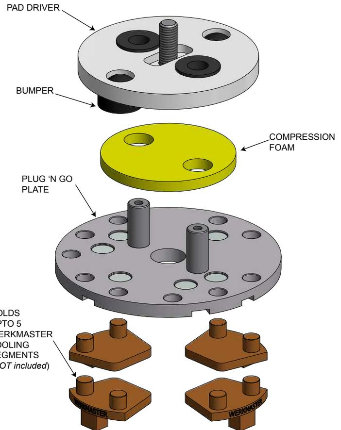
**Just PLUG 'N GO.** When it comes to all WerkMaster Machines, putting on and removing your tooling is a breeze. Strong earth magnets and clip-in tooling save time on any job.
