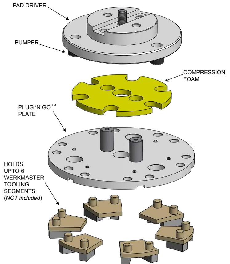
**Just PLUG 'N GO.** When it comes to all WerkMaster machines, putting on and removing your tooling is a breeze. Strong earth magnets and clip-in tooling save time on any job
