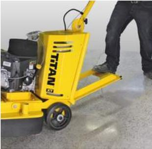
EZ Bak tilt feature allows for operators weighing 135 pounds or more to easily tilt back the machine to change tooling and for transport
